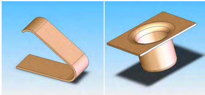
Figure 1 Bent (Left) and Drawn (Right) Features
